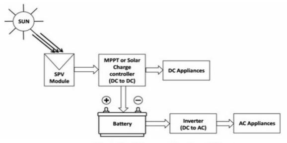
Simple Block Diagram of Standalone SPV system
