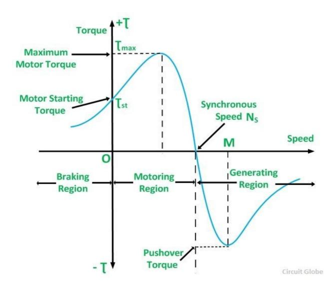
5. Explain the operating principle of squirrel cage induction generator coupled with wind turbine. (APR/MAY2017)
