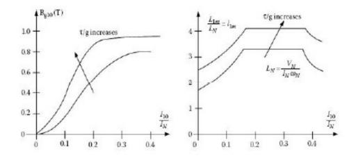
FIGURE Typical airgap flux density (Ber) and magnetization inductance (in per unit [P.U.]) vs. P.U. stator current.
