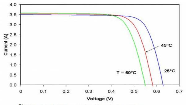
Fig Shows how the I-V curve varies with varying temperature.
