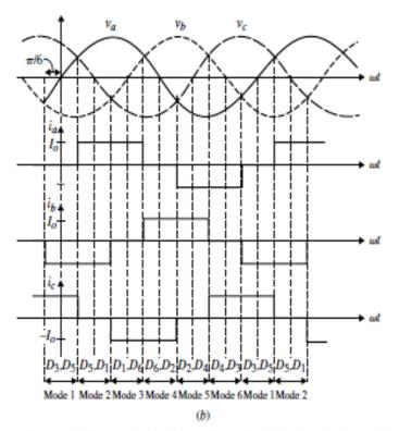
Figure (a) Three-phase bridge rectifier with highly inductive load. (b) Phase current waveforms.
