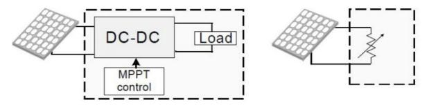
Figure . Basic components of a maximum power pointer tracker
