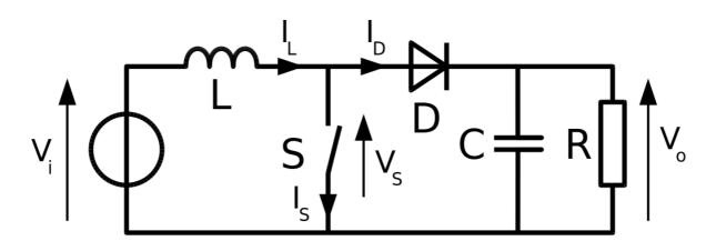
The basic principle of a Boost converter consists of 2 distinct states (see figure below):
