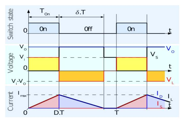
Waveforms of current and voltage in a boost converter operating in discontinuous mode
