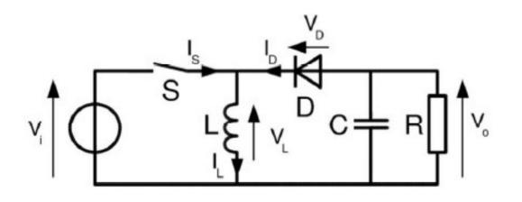
Fig 14 Buck Boost Converter
