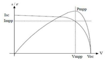
A plot of power (P) against voltage (V) for this device (Fig. 3) shows that there is a unique point on the I-V curve at which the solar cell will generate maximum power. This is known as the maximum power point (Vmp, Imp). Silicon solar cells typically produce only about 0.5 V, a number of cells are connected in series in a PV module. A panel is a collection of modules physically and electrically grouped together on a support structure. An array is a collection of panels (see Figure below).
