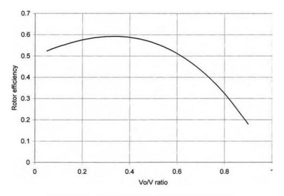
Rotor efficiency vs. Vo/V ratio has a single maximum.
