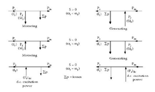
FIGURE Operation modes of wound rotor induction generator (WRIG) at S > 0, S < 0, and S = 0.
