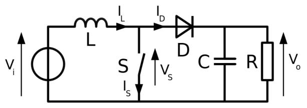
3. What is the function of boost converter in solar photovoltaic system? (APR/MAY2017)
