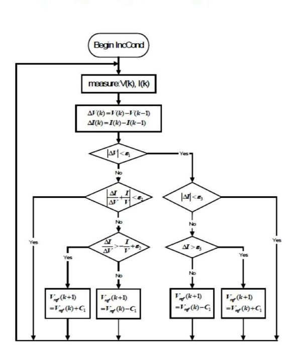
Figure: Incremental conductance algorithm flow chart
