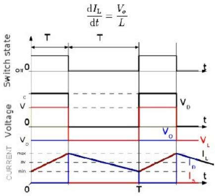
Waveforms of current and voltage in a buck-boost converter operating in continuous mode.
