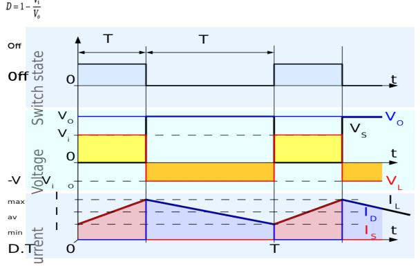
Waveforms of current and voltage in a boost converter operating in continuous mode.
