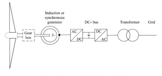
Fig General structure of a full variable-speed WECS
