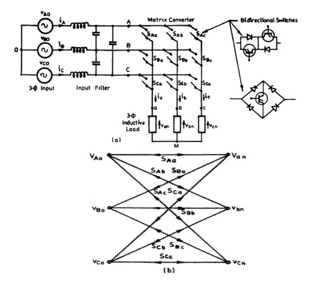
Figure (a) The  $3\varphi$ - $3\varphi$  Matrix converter (b) switching matrix symbol for converter
