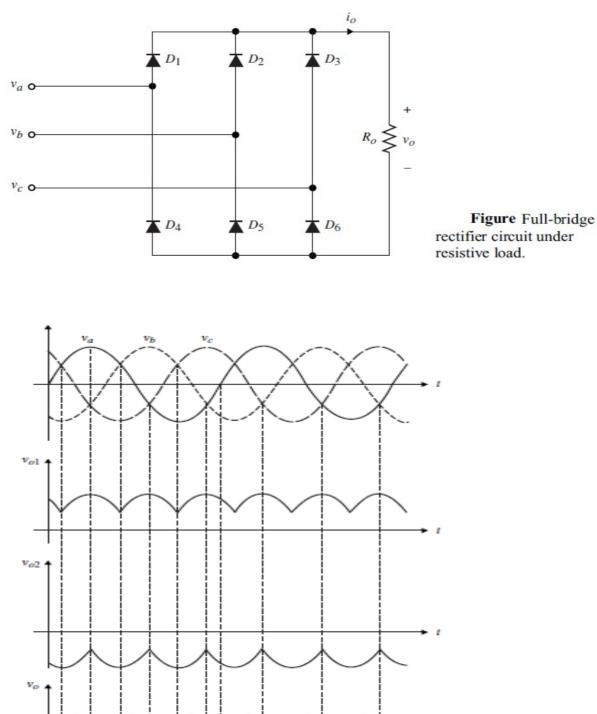
Figure Output voltage waveforms
