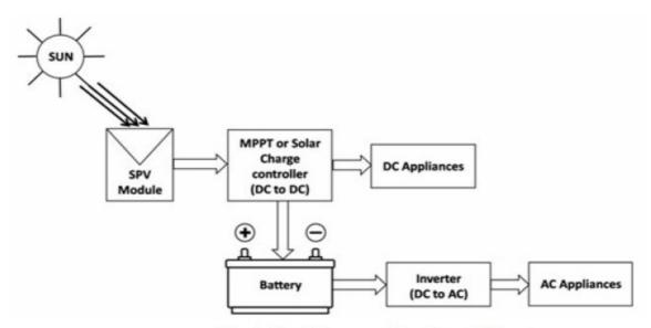
Simple Block Diagram of Standalone SPV system
