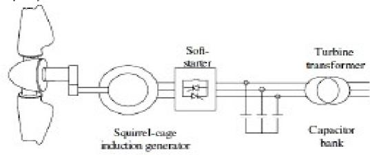
Fig SCIG Connected to Grid
