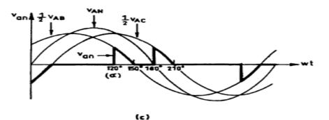
**FIGURE** Output voltage waveforms for a three-phase ac voltage controller with star-connected *R*-load: (a)  $v_{an}$  for  $\alpha = 30^{\circ}$ ; (b)  $v_{an}$  for  $\alpha = 5^{\circ}$ ; and (c)  $v_{an} = 120^{\circ}$ .
