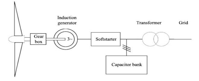
Fig General structure of a fixed-speed WECS
