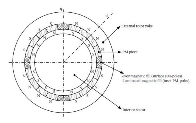
FIGURE Four-pole cylindrical external rotor.
