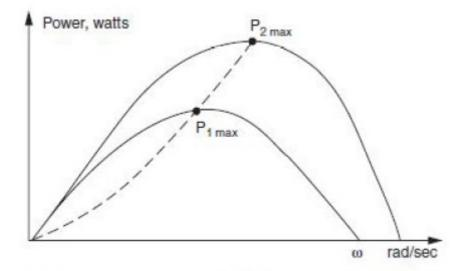
Wind turbine power vs. rotor speed characteristic at two wind speeds, V1 and V2.
