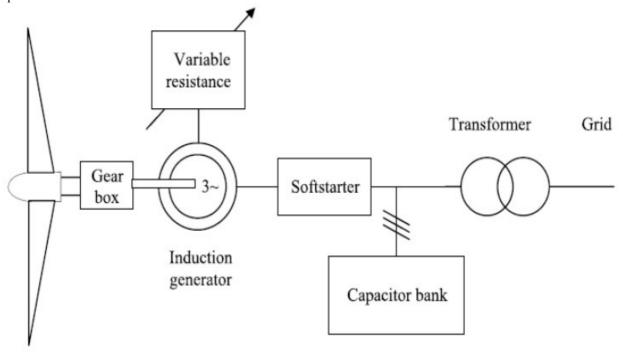
Fig. General structure of a limited variable-speed WECS.
