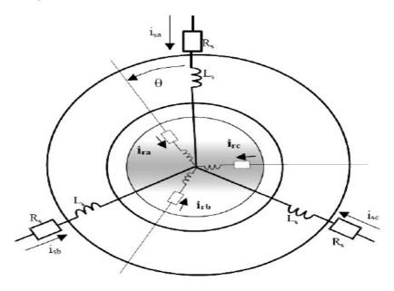
Figure : Induction machine's schematic illustration
