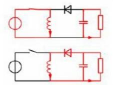
The two operating states of a buck-boost converter: When the switch is turned-on, the input voltage source
