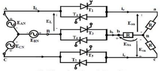
Fig: 1 Three-phase, three-wire Ac regulator
